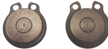
Figure 1: Representation of a correctly (left) and incorrectly (right) mounted retaining ring on a planetary gear.
