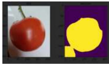
Fig. 8: White or glossy backgrounds create reflections or shadows that negatively affect segmentation.
