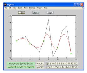
Fig. 5 Bezier spline curve with 3n+1 control points
