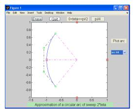
Fig. 6 Approximation of circular arc
