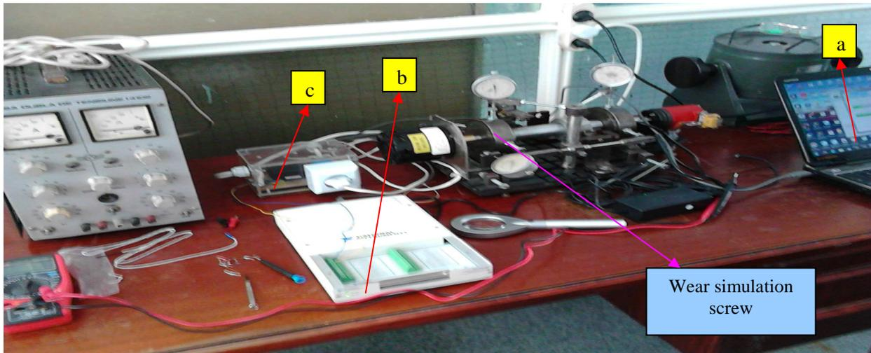
Figure 3. Experimental stand for kinematic chain monitoring
