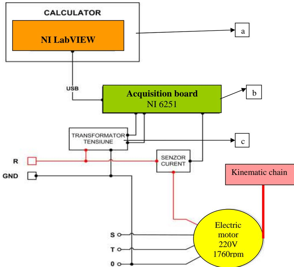
Figure 2. Monitoring system of the kinematic chain parameters
